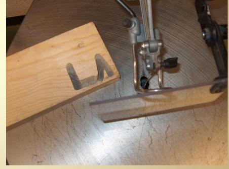
The blade should be installed in a vertical position with the teeth <u>pointing down</u>.
