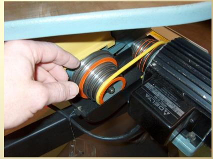
When changing the speed on a variable speed machine it must be running.
