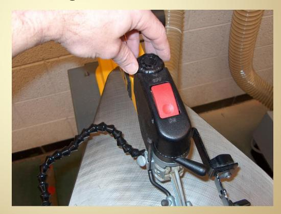
Always check the blade tension before plugging in the machine.
